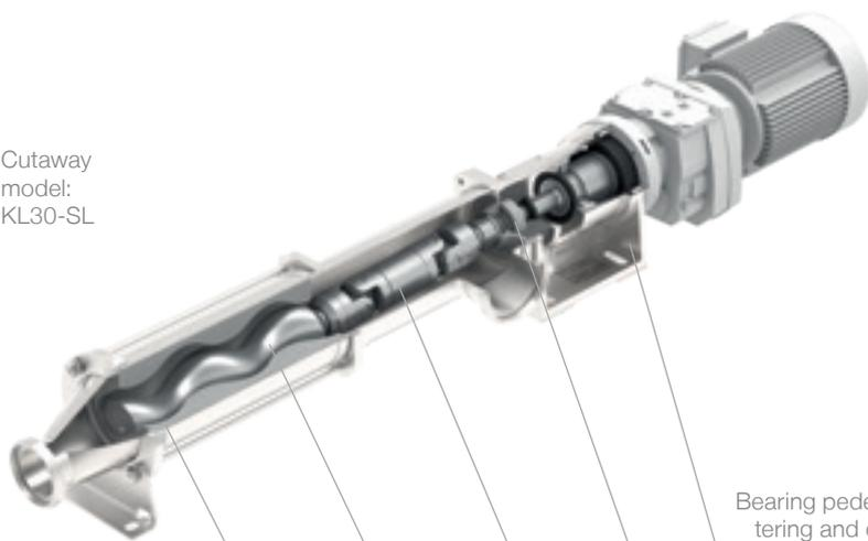
Bearing pedestal with self-centering and direct flange-fitting of the drive unit. This avoids damage to the gearbox.
