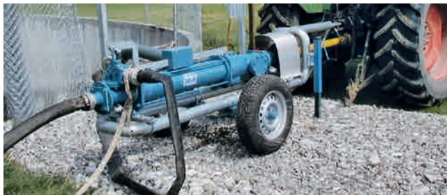
Umbilical system from a liquid manure tank with a pump from the WANGEN GL-series
