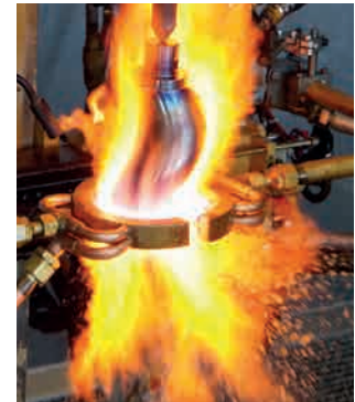
Rotor at flame-hardening process
