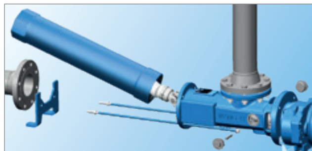
Step 3: Pull the stator and rotor along with the cardan shaft forwards, tip upwards and pull out of the pump housing.
