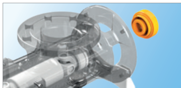
Remove the old seal unit
