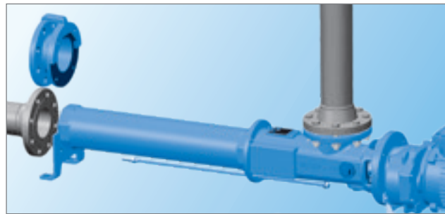
Step 1: Undo the connecting rod on the discharge flange side and push back, remove the discharge flange by lifting up.
