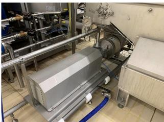
**To summarise**: The combination of the <u>WANGEN Twin NG pump</u> with the <u>Vario Twin NG</u> additional module is an optimum solution for sensitive products in the food sector. High-viscosity and non-free-flowing products, in particular, are transported reliably and energy-efficiently. Sensitive and shear-sensitive textures, like the fine-grained and yet creamy ricotta cheese, are handled gently to guarantee the continuous high quality of the product.
